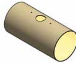
Fig. 63: Drilling two holes (diameter: 13 mm)
