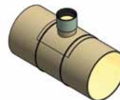
Fig. 66: Placing the saddle
