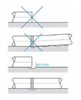
holes must be backfilled with material of a comparable or higher degree of compaction.
